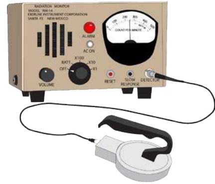
Friskers are one tool used to measure contamination.
