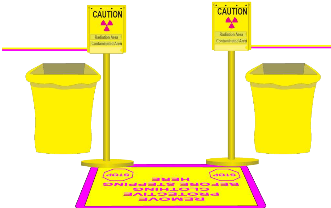
Contaminated area entrance. Notice the Step-Off-Pad, the yellow and magenta rope, and the Contaminated Area signs.
