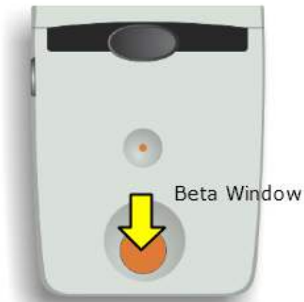
Front of an self reading dosimeter. This one has a beta window.
